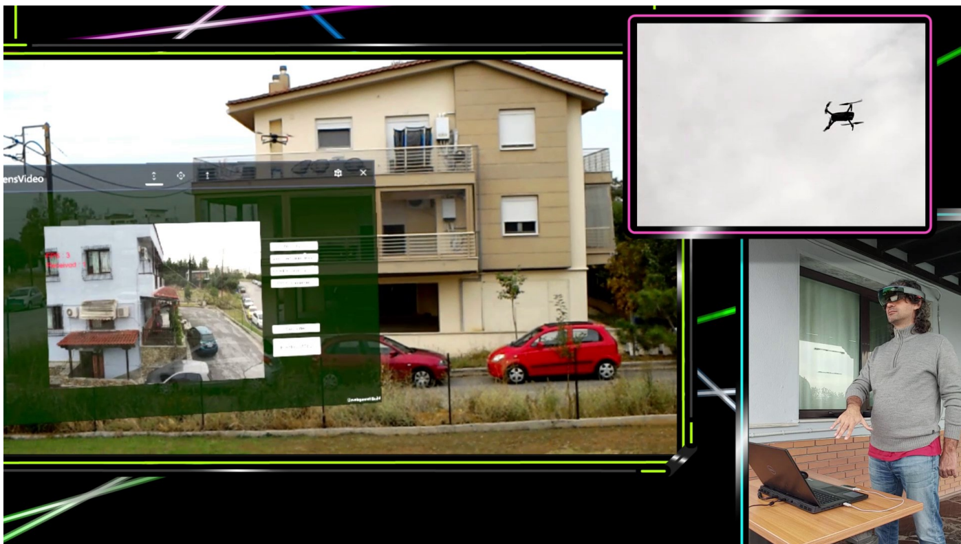
The user (bottom right) can steer the drone (upper right) using hand gestures while watching both the drone and its camera feed (left)
